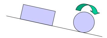
The block's "tendency" will be to slide, but its weight is held there by friction to a certain threshold. However, tilt the plane enough, and the block's "tendency" will exceed the threshold and it will slide:
